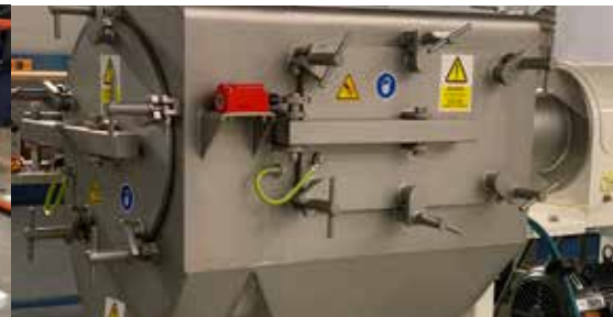
Kek K650CP Pressure Sifter Showing Heavy Duty Hinged Door Clamps
