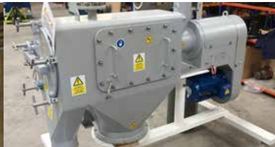
Kek K650CP In-Line Pressure Sifter with Bolted Side Door
